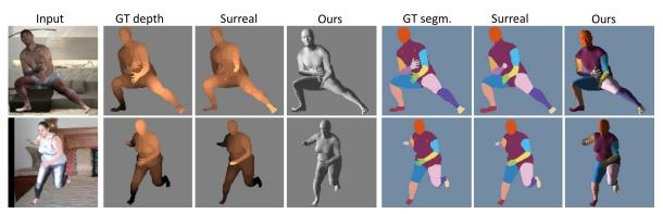
Figure 5: Qualitative comparison of our approach with [52] on recently released SURREAL [52] dataset. Note that [52] trains two distinct conv-nets specific to the task of depth prediction and body parts segmentation. Our method predicts the 3D shape and pose of each body. Depth and body parts segmentation are generated by simply rendering the predicted output shape from camera view.
