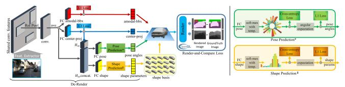
Figure 1: Our network architecture for instance-level 3D object reconstruction. We use ResNet-50-C4 [20] as backbone feature extractor. Layers colored in gray are shared across classes. Render-and-Compare loss is described in §5.3.  $H_{\infty}$  concatenation with RoI features for 3D shape and pose prediction is described in §5.1. Shape and Pose prediction modules are expanded on the right and described in §5.2.
