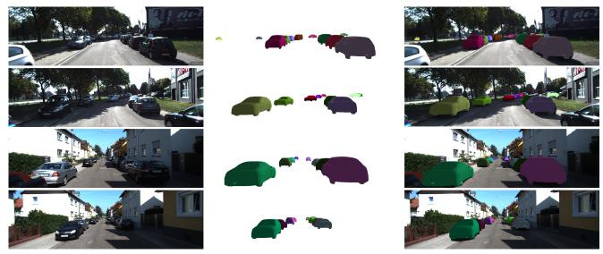
Figure 6: Qualitative demonstration of our approach working on KITTI [13] dataset. Input images are shown in first column, and the corresponding 3D object pose and shape output are shown in second column. Each object instance has been colored randomly. Third column shows the projection of the 3D object instance reconstructions on the input image which demonstrates the capability of producing accurate 2D instance segmentation, which comes for free due our holistic 3D representation.
